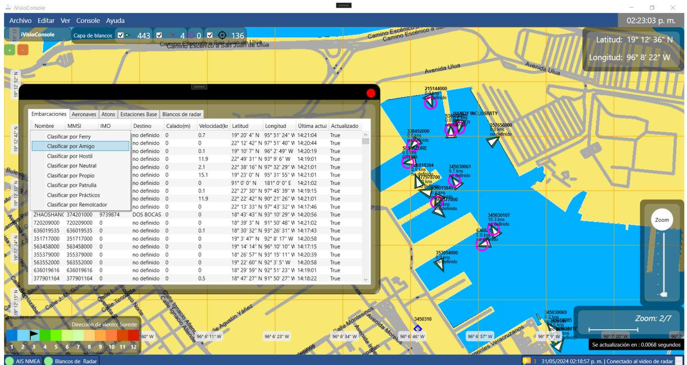
The screenshot shows the iVisioConsole interface. A menu is open over the 'Blancos de radar' tab, listing classification options. The background displays a radar map with various vessel returns and a data table.
