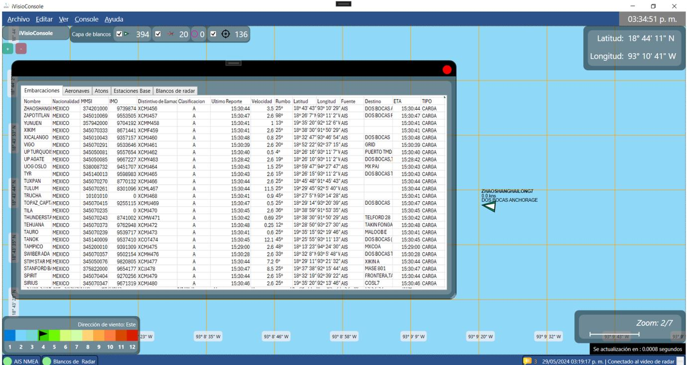
The screenshot shows the iVisioConsole interface with a radar display. A data table is overlaid on the radar, listing AIS targets. The table has columns for Name, Nationality, MMSI, IMO, Call Sign, Classification, Last Report, Speed, True Heading, Latitude, Longitude, Source, Destination, ETA, and Type. A specific target is highlighted with a callout: ZHAOSHANGHAILONG7, 0.0 kts, DOS BOCAS ANCHORAGE.
